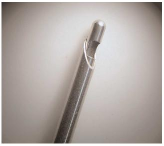
By imposing a welding arc for a controlled period of time, welders can close small diameter tubes to a perfect hemisphere.
