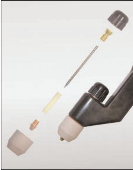
**A plasma welding torch has an intricate internal design to carry plasma pilot gas, shield gas, water cooling hoses, and power cables for plasma pilot arc current and weld current.**
